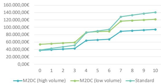
The migration and training costs implied by the change to the M2DC systems in some cases are compensated by the high energy efficiency gain in the long run (at least two-fold). Intelligent monitoring and DC integration highly contribute to these gains. Additionally, the relatively high cost for the basic infrastructure of the M2DC server is compensated by the large amount of microservers that can be integrated into one chassis combined with the embedded communication infrastructure.
