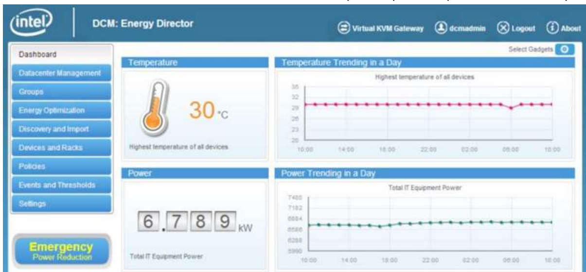
Figure 5: Example screen of modern DCIM software (courtesy of Intel Corp.)
